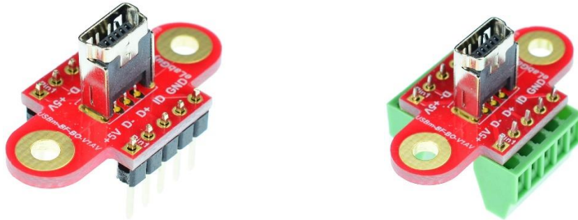
Figure 3: USBm-BF-BO-V1AV Various connections
